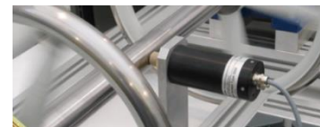
Torque sensor used during the test
