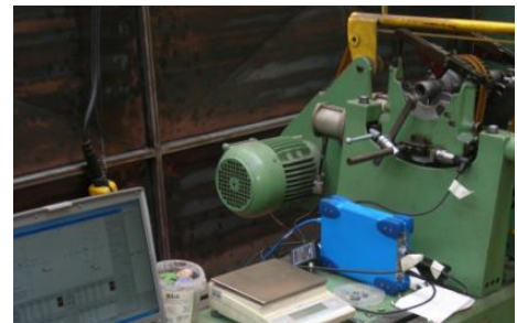
Typical shop balancing set-up with OR34
