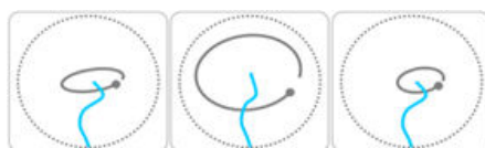
Fig9: Looking at the Full Shaft Motion display along the rotor at 3 bearings
