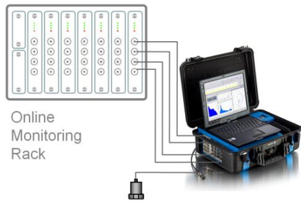
Fig5: BNC/BNC connection to the monitoring rack or direct to sensors
