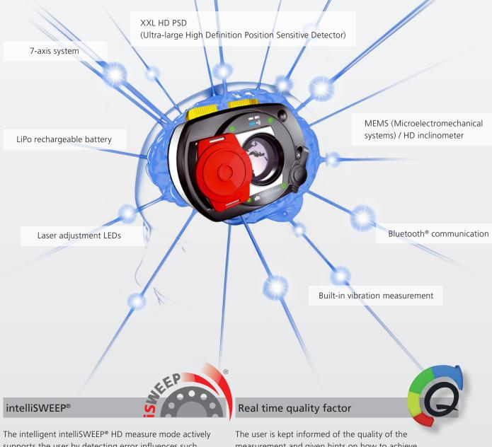
supports the user by detecting error influences such as coupling play, rotational angle or vibration, and automatically eliminating them.
